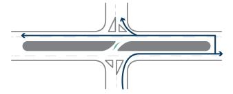
**Diverging** - When one traffic stream splits to form two **Merging** - When traffic streams join to form one **Crossing** - When two vehicles cross paths
